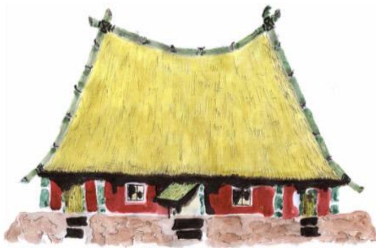
Ancient Vietnamese civilization house built with Rice straw and curved Bamboo tree, created a natural curved roof which is the nature of today's house. (Figure by Dr. Nguyen Thi Thanh)
